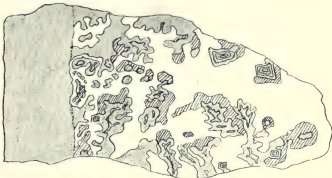
Fig. 30. Diagram of portion of vein from Silver Bar mine, natural size, showing order of deposition. The shaded part represents smaltite-chloanthite intergrowth with chloanthite in the centre of dendritic growths. The hatched part is later niccolite and the white is calcite.
